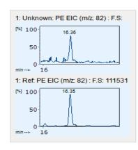
EICs (extracted ion chromatograms) of unknown sample (top) and the reference polymer in the library (bottom)
